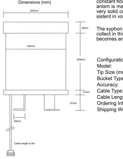
The gauge is also fitted with a syphon to control and maintain a constant flow-rate into the bucket mechanism. The tipping mechanism is manufactured from stainless steel aluminium and is of very solid construction ensuring that tips are accurate and consistent in volume.
