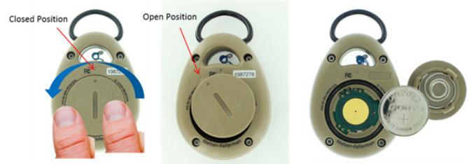
Note: Please inspect the o-ring when opening battery door and ensuring it is clean before replacing door. Also ensure it is properly aligned when closing battery door.
