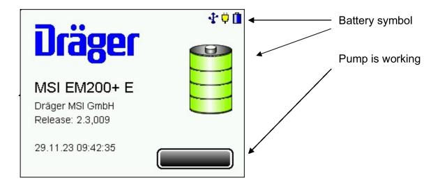
The time and the software version is shown and the battery symbols show the batteries capacity. The bar represents the progress of the run in of the el.-chem. sensors and the progress of the check function.
