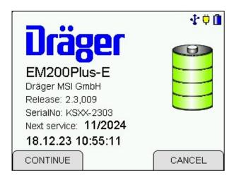
You are informed about the analyser (EM200plus-E), the manufacturer (Dräger MSI GmbH), the date and time when Info Function was called, the version of the firmware (2.3,009), the date of next service (11/2024) and the serial number of the analyser (KSXX-2303).
