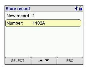
With "F" (SELECT) you may call "Selection and Input of Engine Number" (see 10.). This function makes it possible, to alter the displayed engine number, to select another exist-ing number or to create a new engine number. After this the former display screen is called.
