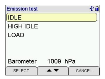
"Barometer" is the absolute ambient pressure, not calculated regarding to any reference (sea level etc.), like it is done for meteorological values. The altitude of the level in a mine, where the MSI EM200 E is used, influences the absolute pressure of the ambient air.
