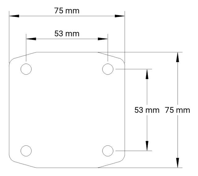
Use M4 screws for fixing the button to the installation surface.
