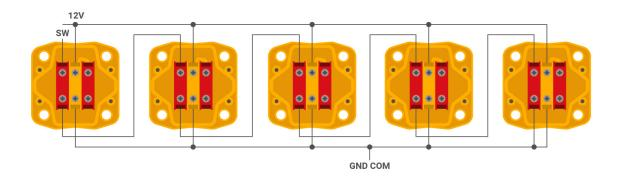
Connection schema for multiple pushbuttons.
