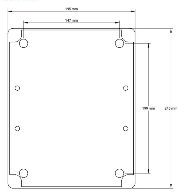
Use M5 screws of appropriate length to fix the enclosure to the mounting surface.
