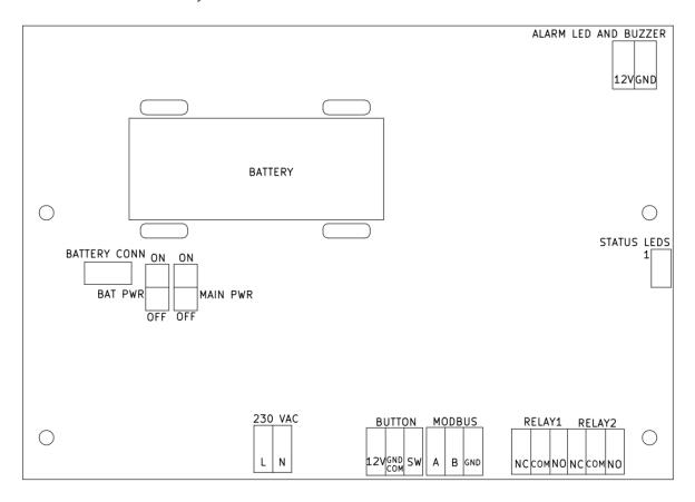
Connector placement on the main board
