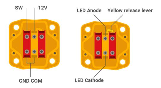
Connection schema for the emergency pushbutton
