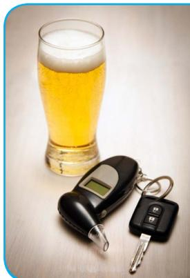
Cheaper personal breathalysers, such as those sold at auto supplies stores, use semi-conductor sensors which do not match the accuracy offered by fuel cell sensors.
