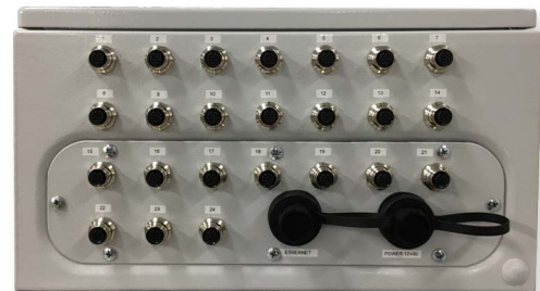
Measure up to 24 inputs - Expandable to 320
